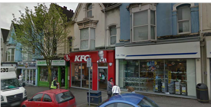
Left: This row of shops shows how fascia signs can be staggered/stepped to provide a relatively uniform transition along a terrace of shops on a sloping street/hill.
