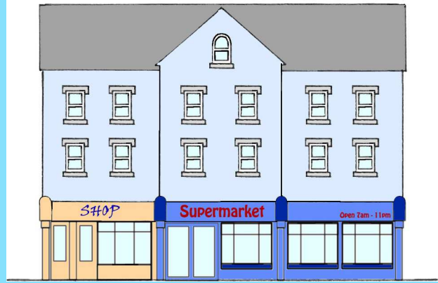
A consistent fascia relates to the adjacent shopfront and the rest of the building.
